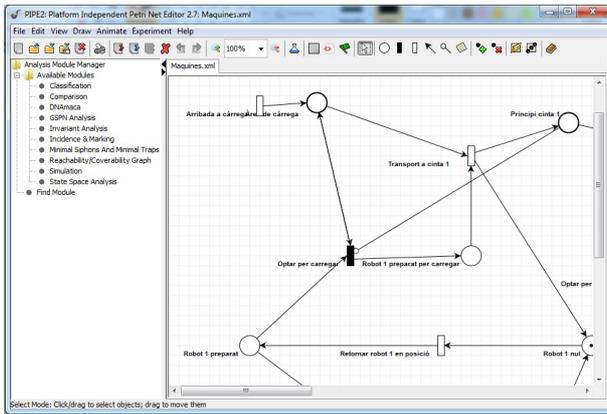
Figure 3: PIPE 2.7 GUI with the analysis modules on the left side
